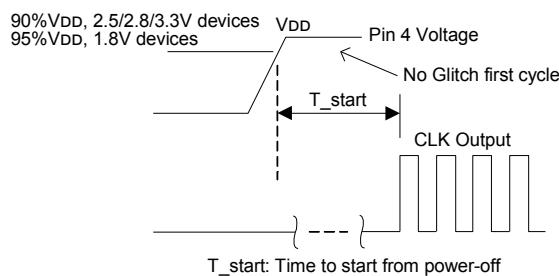
FIGURE 4. STANDBY RESUME TIMING (ST MODE ONLY)
